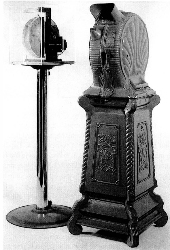
1.12 At the right, a Mutoscope, a penny-in-the-slot machine with a crank that turned a drum containing a series of photographs. The stand at the left shows the circular arrangement of the cards, each of which flipped down and was briefly held still to create the illusion of movement.
